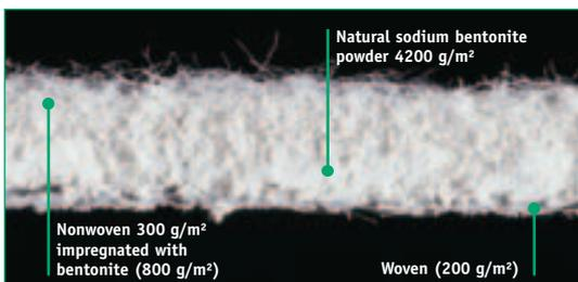
In 1987 **NAUE** developed **BENTOFIX®**, a bentonite geosynthetic clay liner.
