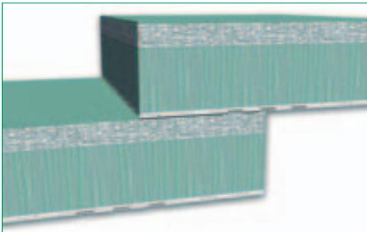
The key to the success of **BENTOFIX®** lies in the manufacturing process. Natural sodium bentonite is encapsulated within the void spaces of two geotextile layers in a special needle-punching process (produced under patent number EP 0 278 419 by **NAUE**).
