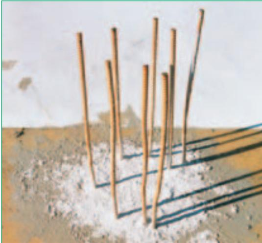
The bentonite powder (supplied in 30-kg-bags) is mixed with water in the ratio of approx. 4 parts water and 1 part sodium bentonite. This transforms the dry bentonite powder into a soft smooth gel-like consistency allowing easy handling and moulding for repairs and additional seals.
